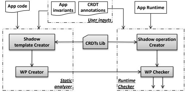
Figure 1: Overview of SIEVE. Shaded boxes are system components comprising SIEVE. (WP stands for weakest precondition.)
