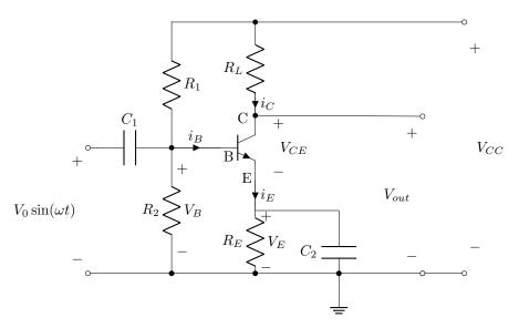
If you recall JEE Physics, this is a circuit diagram of an npn transistor used as an amplifier. Try your best to match this circuit. We have used the American voltages convention. It is alright if you can't get the dimensions to match. What is important is that you know how to use circuitikz to draw circuits with the components used above, and mark voltages and currents.
