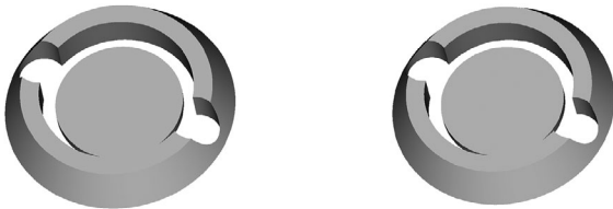
Figure E7: Speaker Grill (ground truth on the right). The mesh error is 3.78%.
