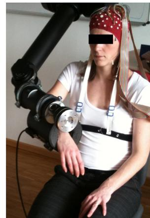
Fig. 1. A robot arm is attached to the patient’s forearm and it may move the patient’s forearm with the elbow as the single degree of freedom (DoF). The resting position, maximum extension and maximum flexion of the robot arm can be adjusted depending on the patient (adapted from [20]).
