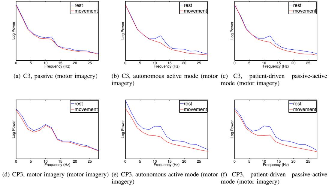
Fig. 4. **Power spectra of the electrodes C3 and CP3 for healthy subjects:** Power spectra in movement periods and the rest periods for the electrodes C3 and CP3 in the frequency band 2–30 Hz for motor imagery (i.e., no robot neither real movement), the autonomous active mode and the patient-driven passive-active mode (adapted from [20]).
