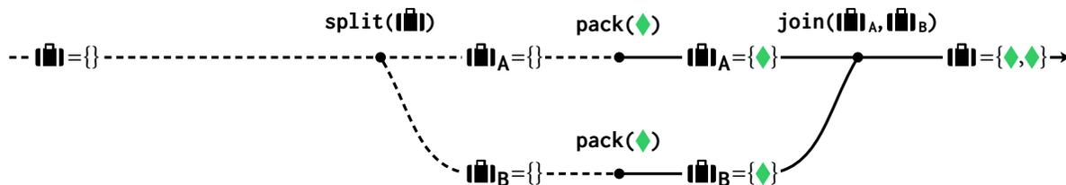
(b) Baggage is empty when the execution branches. Both branches of execution encounter distinct events that pack a tuple; however, the tuples happen to have the same value (both ♦). When the execution joins, the two identical tuples must both be retained, because they capture different happened-before relationships.
