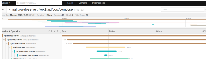
Fig. 1. Trace visualisation from Jaeger [2], an open-source DT tool. The trace depicts a ComposePost API call to the DeathStar social network application [8], a small-scale open-source microservice benchmark.
