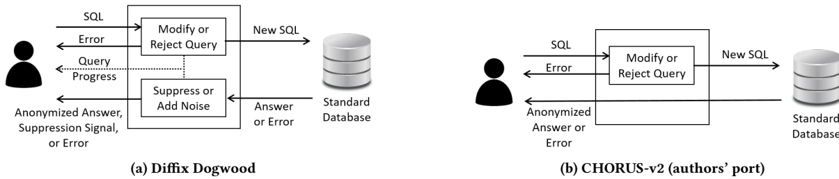
Figure 1: Operation of Diffix Dogwood and CHORUS-v2 systems. Both systems operate as a proxy in front of a standard back end database.
