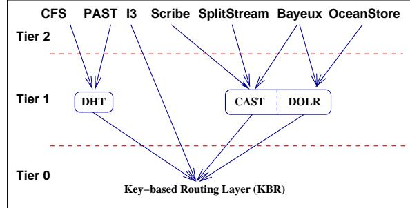
Figure 1: Basic abstractions and APIs, including Tier 1 interfaces: distributed hash tables (DHT), decentralized object location and routing (DOLR), and group anycast and multicast (CAST).
