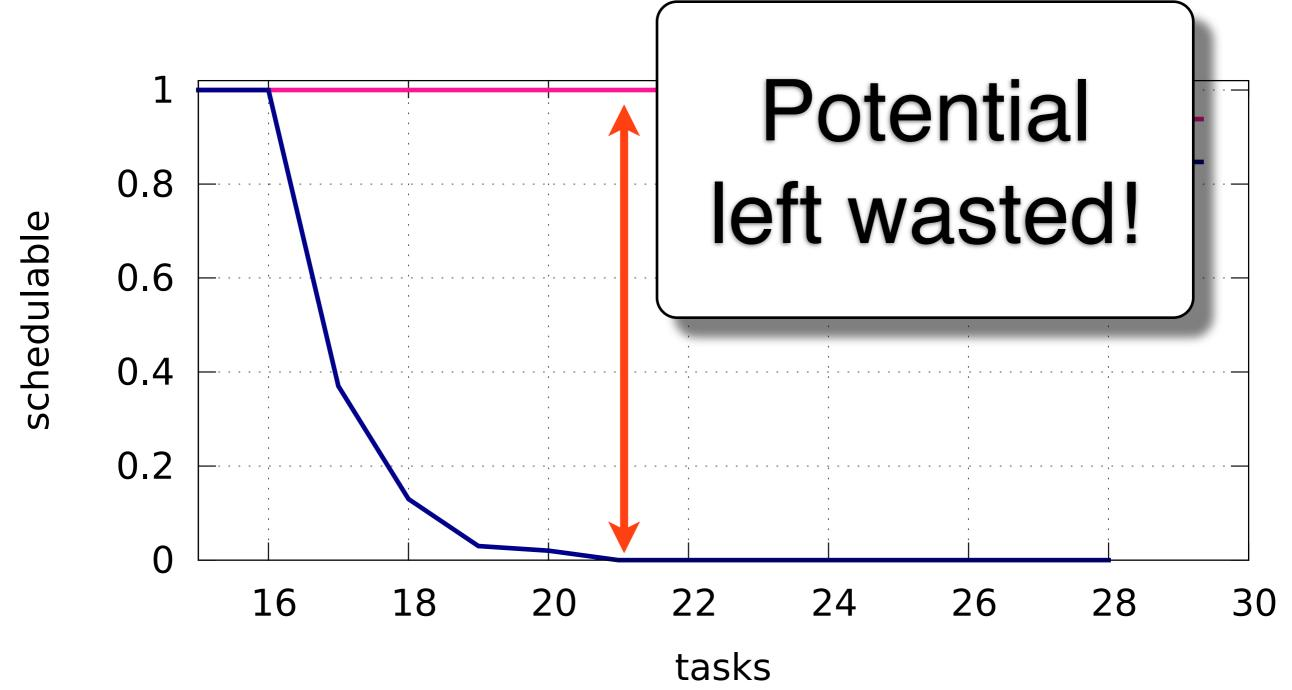
8 processors, 16 resources, critical section lengths in [1us,100us], periods in [3ms,33ms], 10% average task utilization
