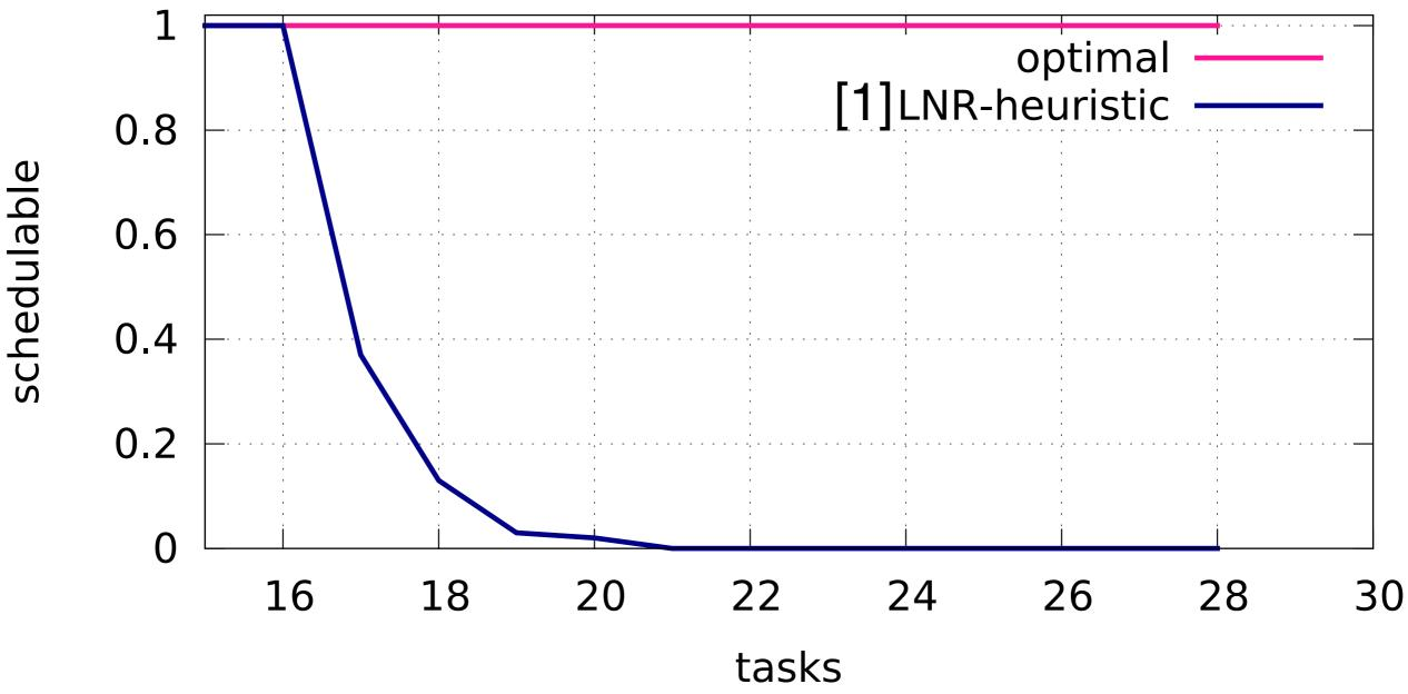
8 processors, 16 resources, critical section lengths in [1us,100us], periods in [3ms,33ms], 10% average task utilization
