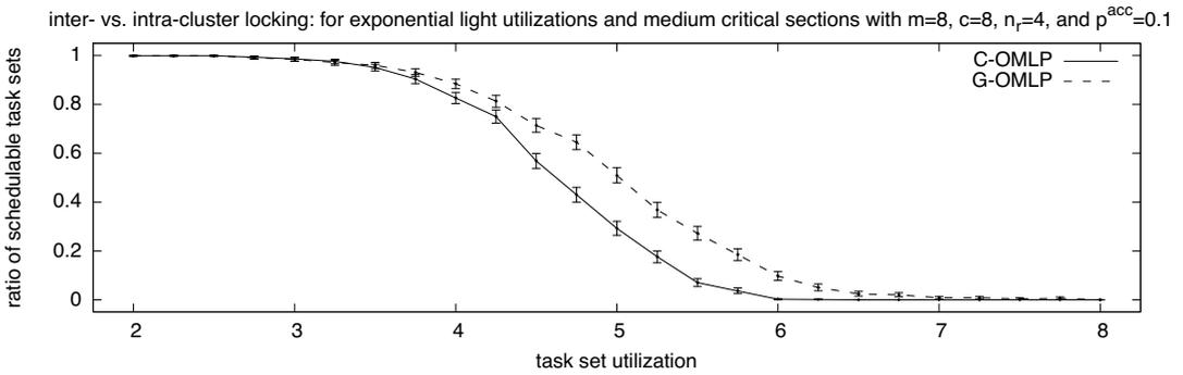
(b) Under global scheduling ( $m = c$ ), the global mutex protocol is not limited by partitioning constraints**Fig. 12** Comparison of the OMLP's mutex protocols for global and clustered scheduling under C-EDF scheduling
