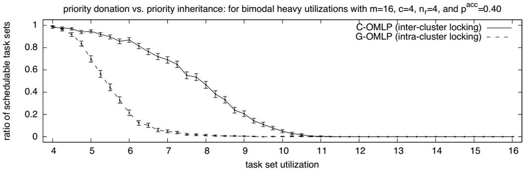
(b) Schedulability is low under the global OMLP because the intra-cluster locking constraint cannot be satisfied for large  $n$ **Fig. 13** Comparison of the OMLP's mutex protocols for global and clustered scheduling under C-EDF scheduling in the case of heterogeneous task sets
