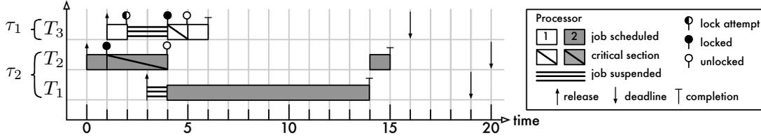
Fig. 8 Pi-blocking of independent jobs under the clustered OMLP and P-EDF scheduling on  $m = 2$  processors with  $c = 1$
