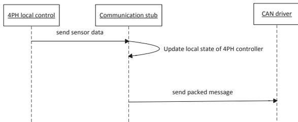
Figure 4. Interaction diagram for sending a CAN message.
