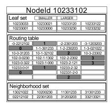
Fig. 1. State of a hypothetical Pastry node with nodeId 10233102, b = 2. All numbers are in base 4. The top row of the routing table represents level zero. The neighborhood set is not used in routing, but is needed during node addition/recovery.
